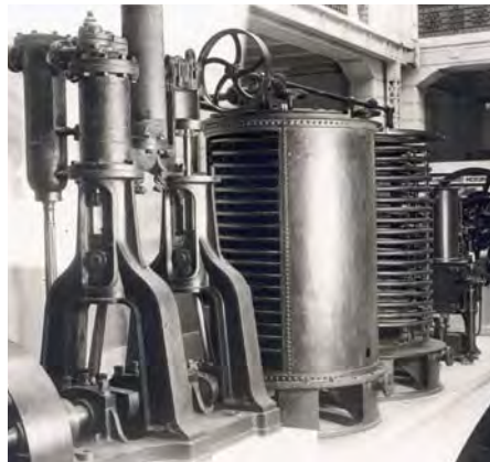
Fig. A.1–3 Linde refrigeration machine from 1877
